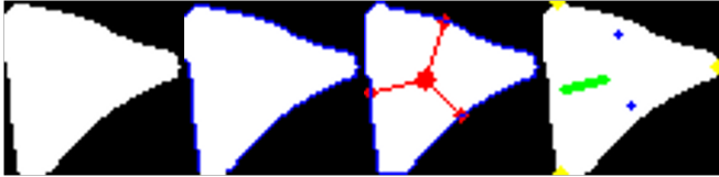
Fig. 2. Object masks obtained from the image segmentation. The proposed method first obtains the contour of the mask (in blue). It then finds the closest point from the centroid on each edge of the contour (in red). The grasp point is the contact point with minimum distance (in green).
